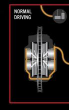
Without Dual-Grip™ shims, brake pads may drag on rotors and create DTV
